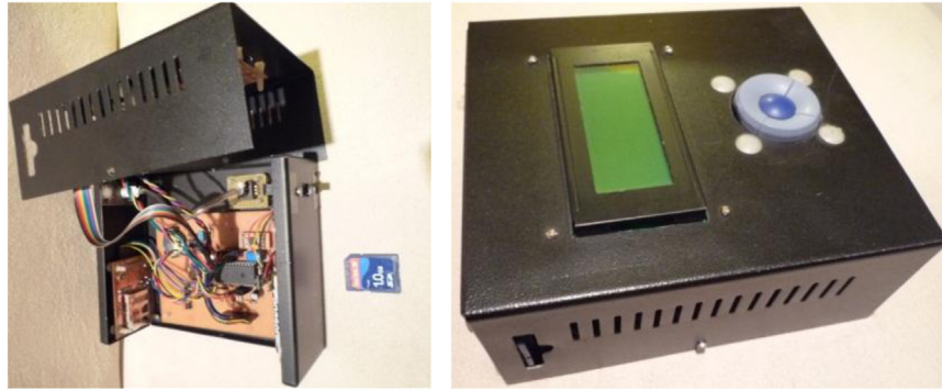
Fig. 5 – Apparatus developed to measure the pressure inside the skin expander.
