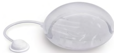
Fig. 3 Tissue expander to grow skin for defect correction in reconstructive surgery. Typical applications are birth defects, burn injuries, and breast reconstruction. Devices consist of a silicone elastomer inflatable expander with a reinforced base for directional expansion, and a remote silicone elastomer injection dome. Courtesy of Mentor Worldwide LLC.
