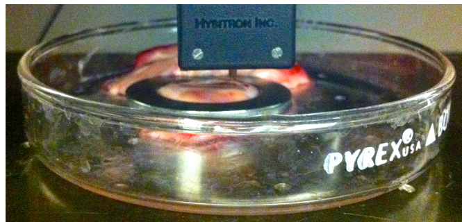
Figure 2: Experimental setup. A 5mm thick coronal slice of freshly harvested brain tissue is placed in a 100mm-diameter petri dish and mounted underneath the force transducer of the TriboIndenter™. The surface of the sample is continuously hydrated with saline solution. A 12mm-diameter washer marks the indentation region and stabilizes the sample. A circular flat punch of 1.5mm diameter ensures a homogenized specimen response.
