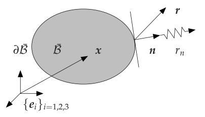
definition of contact heat flux  $q_n$  in analogy to Cauchy's postulate, lemma and theorem originally introduced for the momentum flux in §3.1.2
