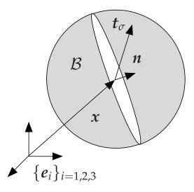
the traction vector  $t_{\sigma}$  at a point x can be expressed exclusively in terms of the point x and the normal n to the tangent plane to an imaginary surface passing through this point
