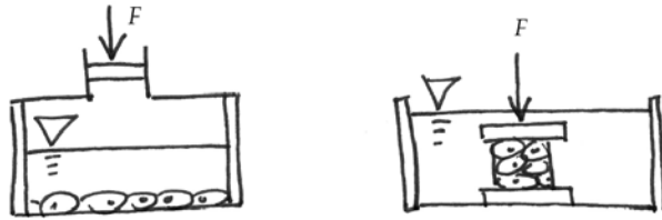
Figure 6.2: Hydrostatic and uniaxial compression devices compressing plain cells and cells in a matrix.
